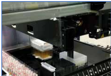
Alternatively, thin metal tips can be used for filling and air inclusion-free mixing.
